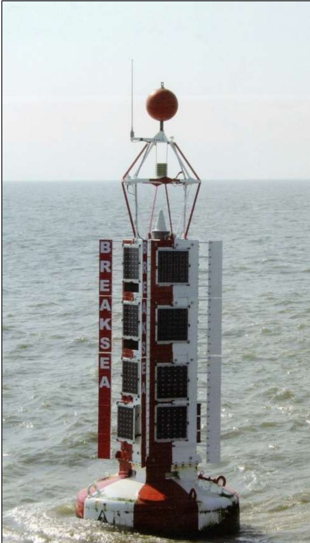
Fig.86 Large solar powered buoy with Racon, LED lantern and AIS installation.
