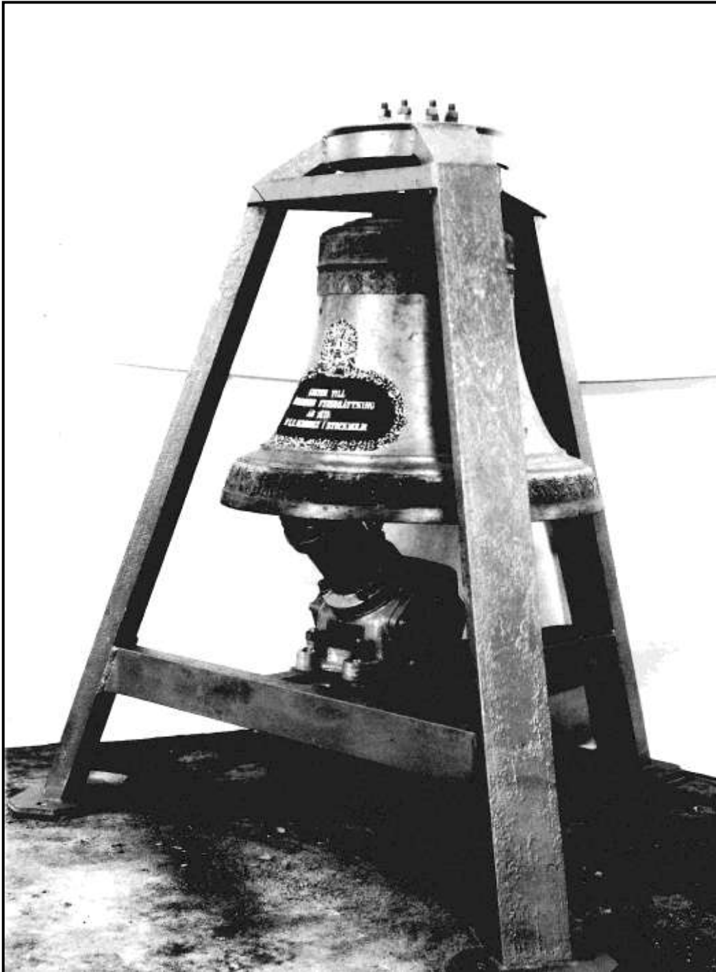
Fig.72 AGA carbon dioxide fog bell
