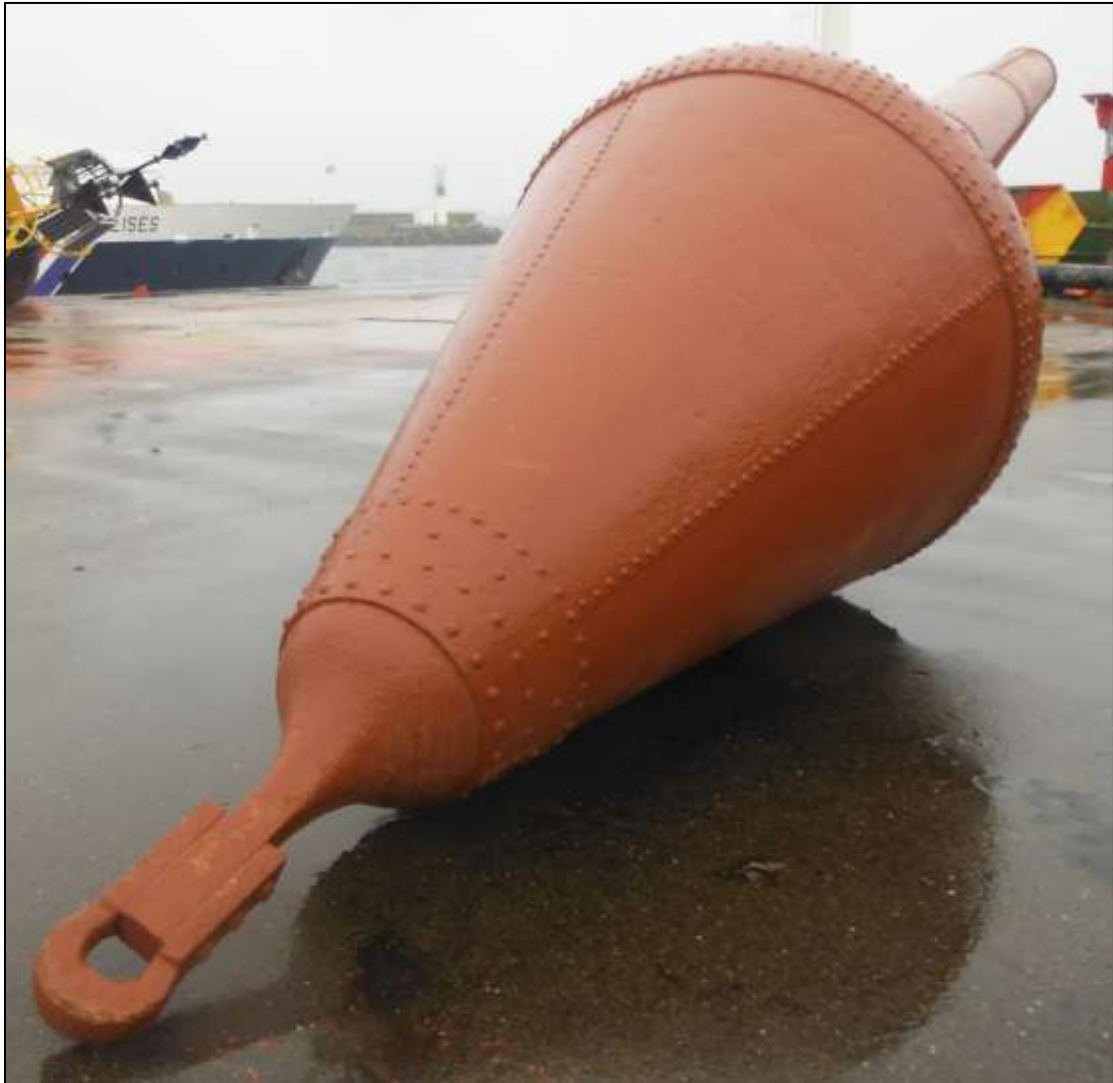
Fig.33 French riveted iron buoy, 1880s design.
