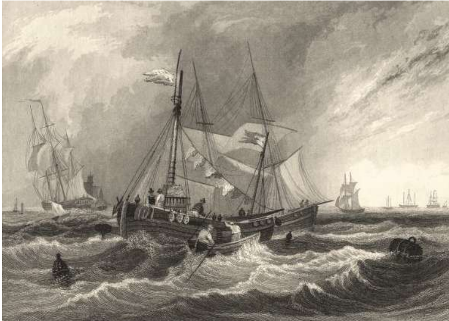
Fig. 18 Nore Lightvessel in 1830 The lantern encircles the mast and would be hoisted up the mast at night.
